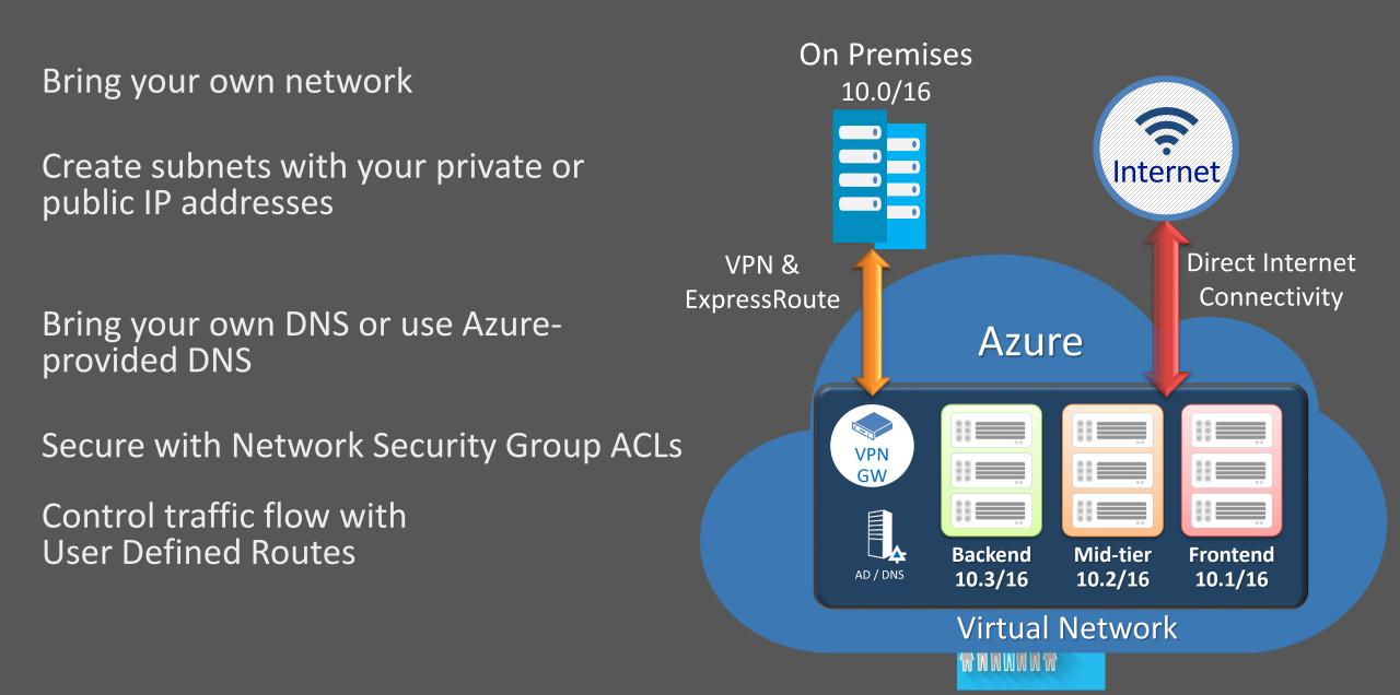
Segment network to meet security needs Can protect Internet and internal traffic Enables DMZ subnets Associated to subnets/VMs and now NICs ACLs can be updated independent of VMs
